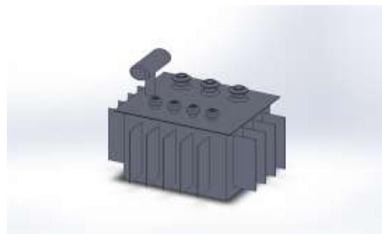
Fig 6: Distribution Transformer model using Solid works software
